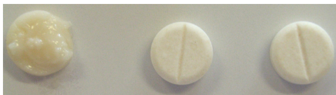
Figure 3: Appearance of sodium valproate tablets after 21 days of storage at accelerated (40°C; 75% RH) (left), refrigerated (2–8°C) (middle) and controlled room temperature (25°C) (right) conditions.
